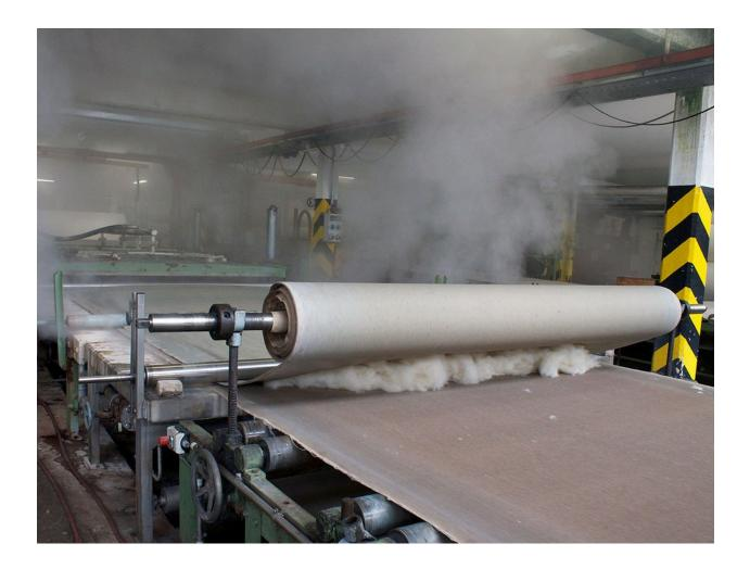
The performance of felt material in sound attenuation, vibration isolation and shock absorption is based on the unique properties of wool felt fibers in a non-woven matrix of various densities. Shock implies a single, sharp displacement that may or may not excite resonant vibration. In general, periodic oscillation up to about 50 cycles is considered vibration; above that frequency it is considered sound or, if it includes a mixture of frequencies not harmonically related, noise.
